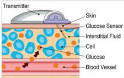
**Figure 3: FGM Sensor and Reader**
